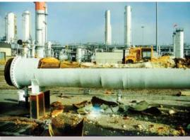
Photo 6: Deformed condenser shell.
